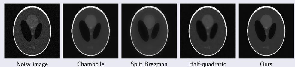
Figure : Denoising experiment on Phantom image corrupted with noise s.d.  $\sigma = 30$ . All results except ours suffer from over-smoothing and, furthermore, some image features have disappeared. On the contrary, our result looks clear and best approaches the ground truth.
